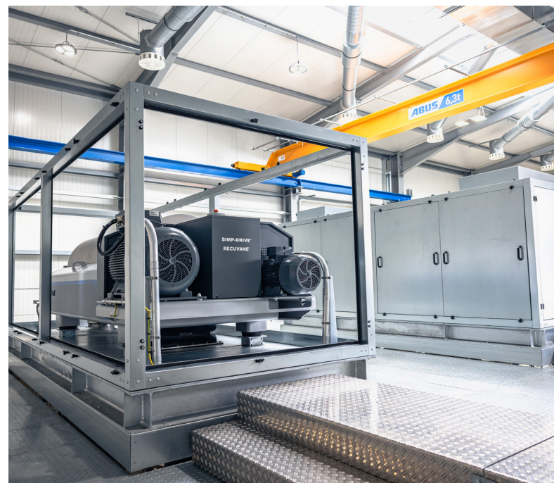
The two X5Es from Flottweg - without (front) and with (back) acoustic hoods.
